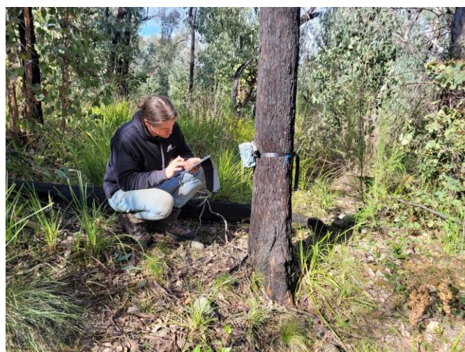
Figure 4. Typical camera trap set up, with the camera fastened to a tree, approximately 50cm off the ground.
