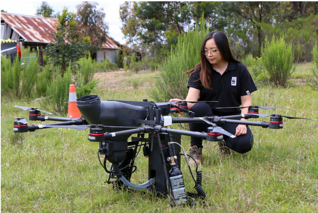
AirSeed Technologies demonstrate their seed-dispersing drones at a property at Marulan. © WWF-Aus / Paul Fahy
